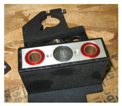
Once the bearings are shimmed or replaced re attach the parts in the reverse order from above.
