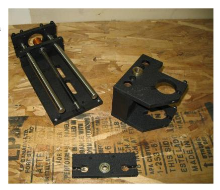
4. Use the same 1/8" wrench to remove one of the slide block end plates. This will expose the bearings.
