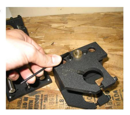
5. The red pieces are the bearings that slide on the rod. If you are experiencing play in the height control you will need to see if the bearings can move in the slide block or if the bearings are loose on the linear rods.
