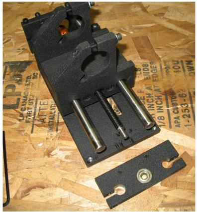
3. Turn the lead screw until the mounting block slides free from the rails
